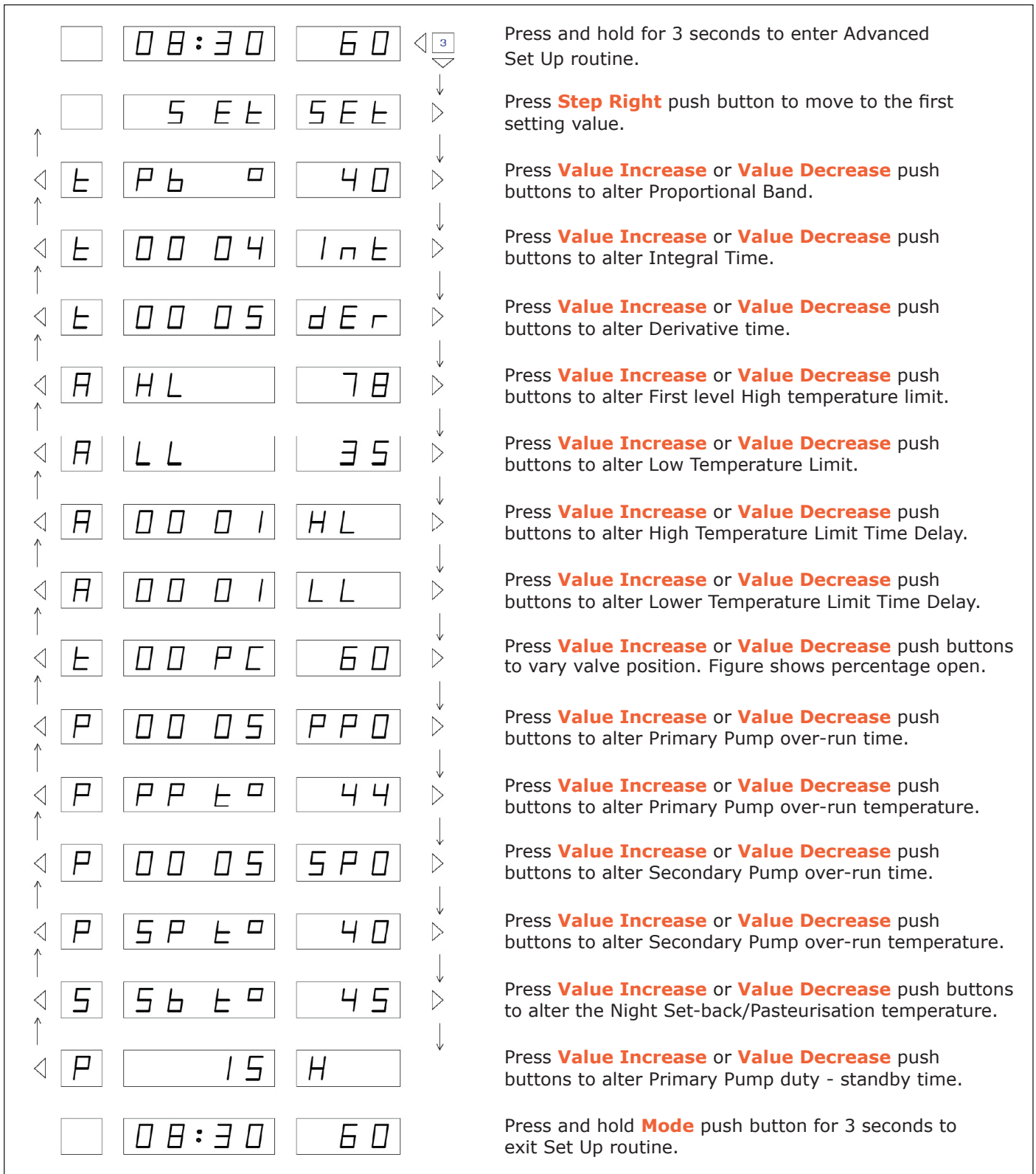
Figure 3 - Advanced Set Up
